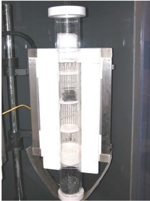
Figure 2. Sulfuric Acid Exposure Rig.
