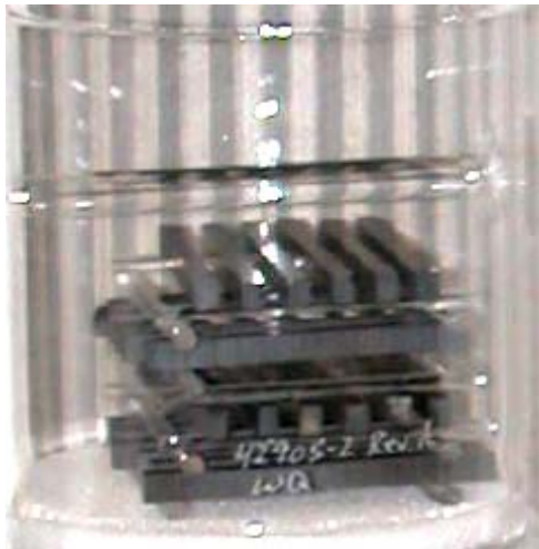
Figure 3. Bend bar arrangement in small sample cups.
