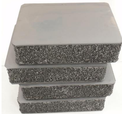
Figure 5 Millimeter scale foam bonded to dense layers.
