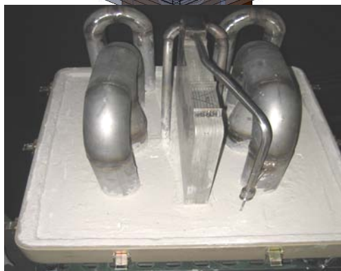
Figure 5: As built TARDEC reformer
