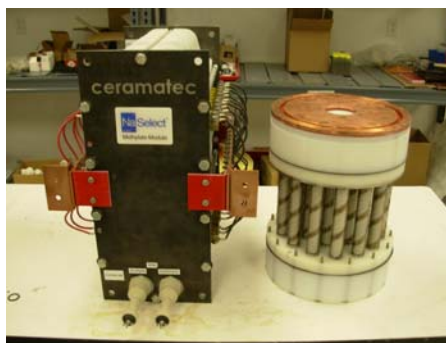
Figure 7: Planar type NaSICON membrane electrolysis stack on left and Tubular NaSICON membrane bundle on right
